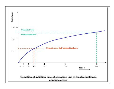
This diagram illustrates the importance of concrete cover. The concrete cover represents a form of "barrier protection" through which the corrosive elements must pass before attack on the reinforcement can commence.
