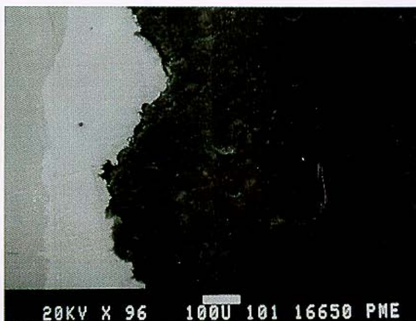
Figure 10 – SEM Photo of Bar/Coating/Concrete Interface of Bar #1
