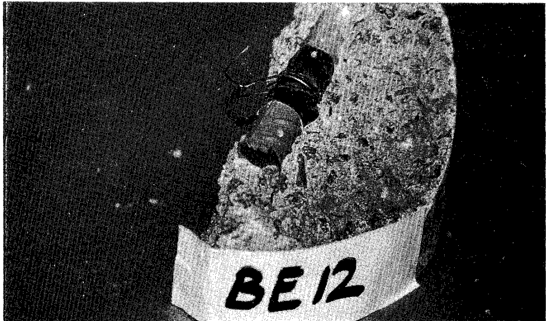
Plate 12: Sample BE12: Epoxy Coated - Salt Fog - 132 Days. Corrosion activity at repaired end of bar with 32 mm cover.
