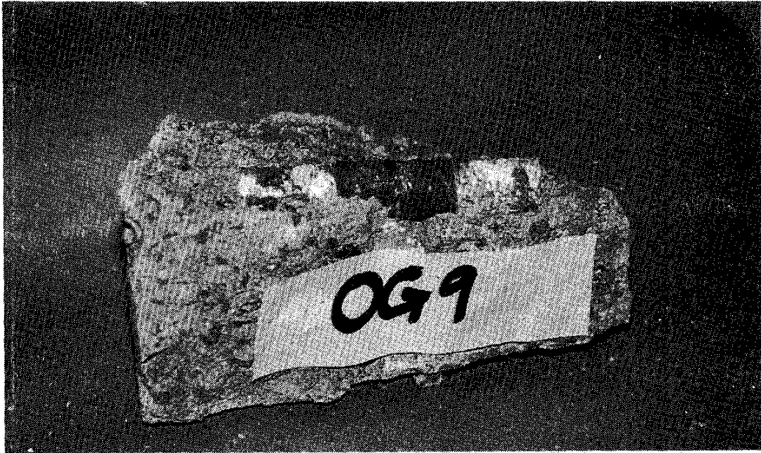
Plate 9: Sample OG9: Galvanized Steel - Wet and Dry - 132 Days. White zinc reaction products on bar with minimum cover at ends of 32 mm.
