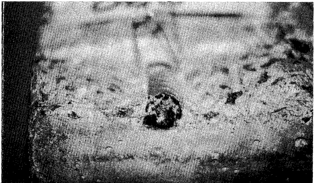
Plate 6: Sample OE8: Epoxy Coated Steel - Wet and Dry - 98 Days. Corrosion at unrepaired exposed end of longitudinal bar.
