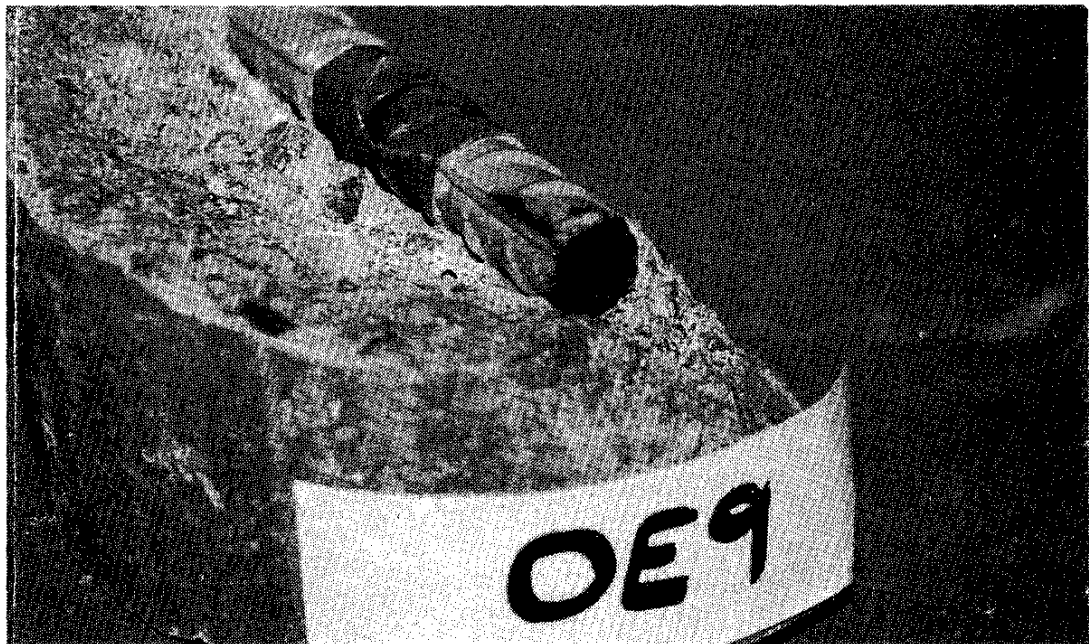
Plate 14: Sample OE9: Epoxy Coated - Wet and Dry - 132 Days. Corrosion at unrepaired end of bar with 32 mm cover also showing localized attack along the bar away from cut edge.
