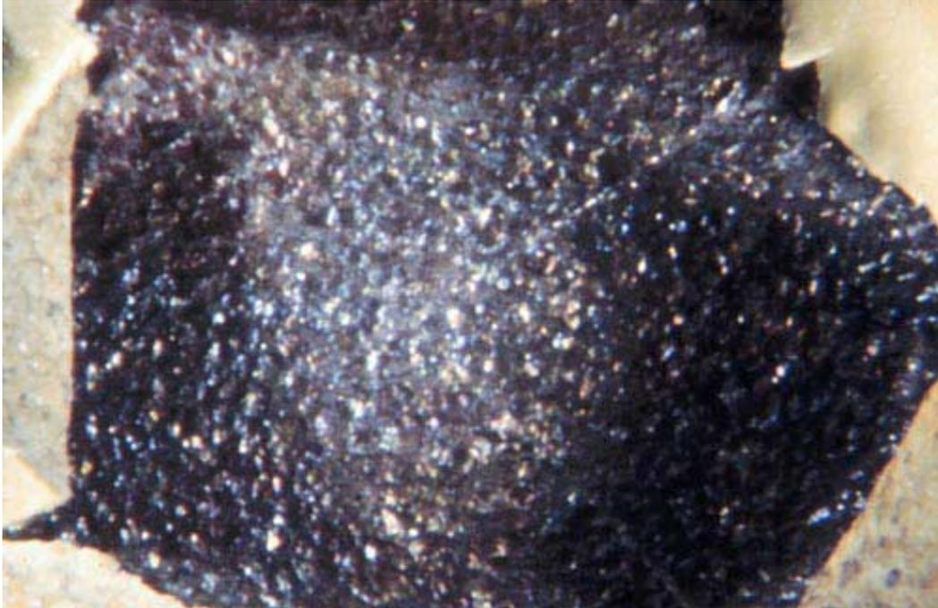
Figure 44. Black, Shining Steel Surface Underneath Coating.
